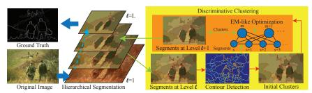
Fig. 2: Our proposed hierarchical image segmentation framework.
